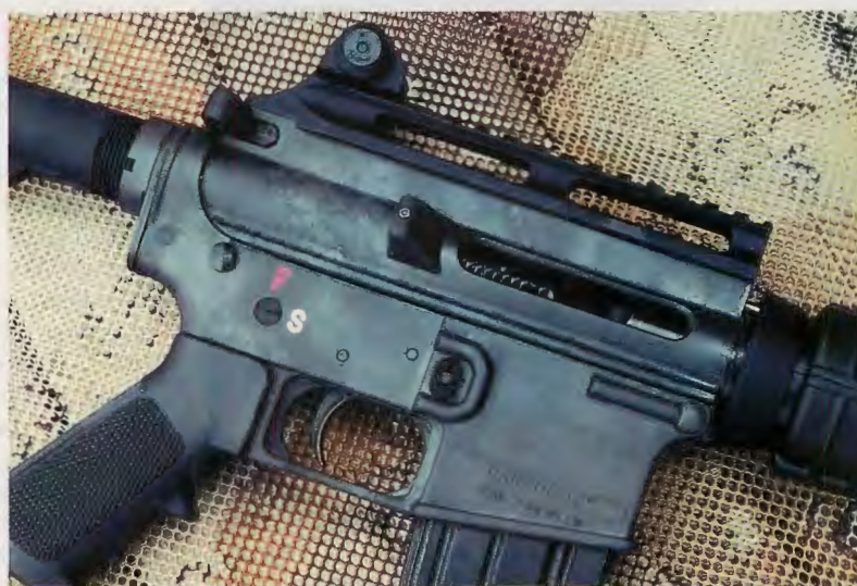
Having a raised rail platform, the Carbon 15 has no forward assist, and differs from a standard AR-style receiver in other details, but is otherwise interchangeable.
